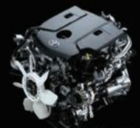
NEW - 2GD-FTV, Efficient & Powerful 2.4L Turbo Diesel Engine
