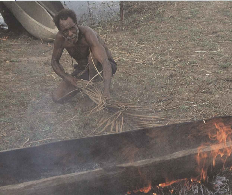
Above Charring process is also used to seal and harden the exterior. right Putting the finishing touches on a new canoe.
