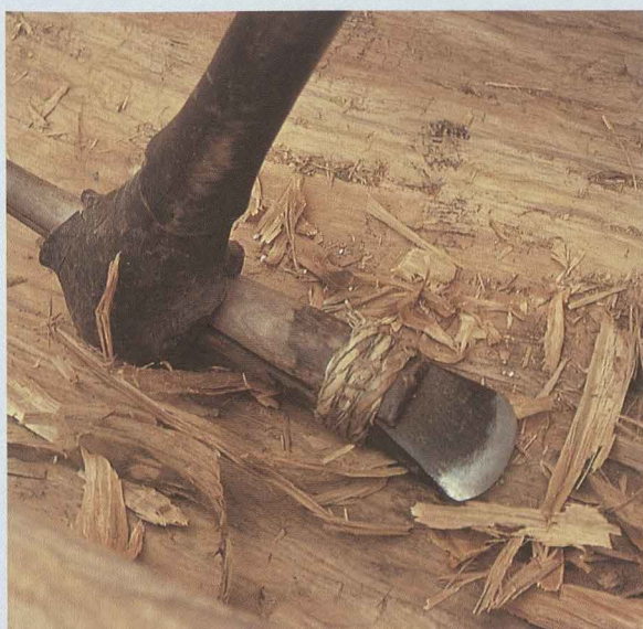
Above Adze head can be rotated to cut at any angle. right Chopping out the interior of a log.
