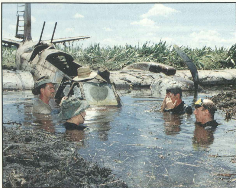
Cool conference in a hot climate — members of the recovery team decide what to do next. The zero visibility in the swamp and the laminated safety glass in front of the pilot are clearly evident.
