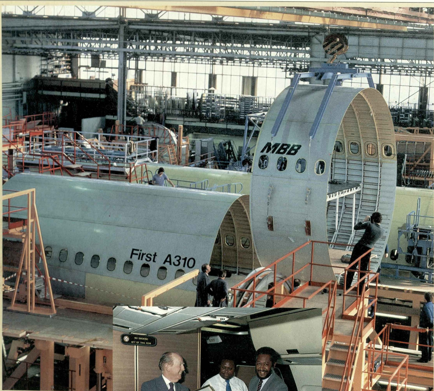
Above: the fuselage of the Airbus A310 comes together at the Airbus Industries factory at Toulouse in France
