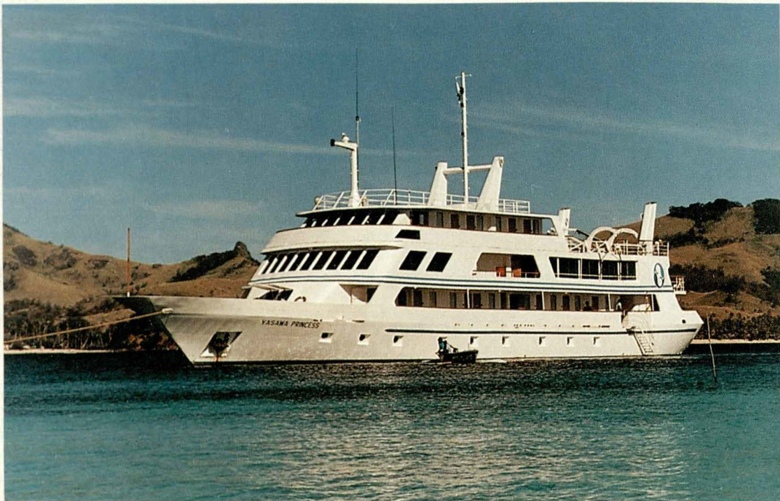
"The magnificent 54 metre Yasawa Princess recently built in Suva for Blue Lagoon Cruises. The Yasawa Princess has been treated inside and outside with Dimet high performance zinc silicate, epoxy, vinyl and anti-fouling marine coatings. Application by Maxlane Engineers Ltd."
