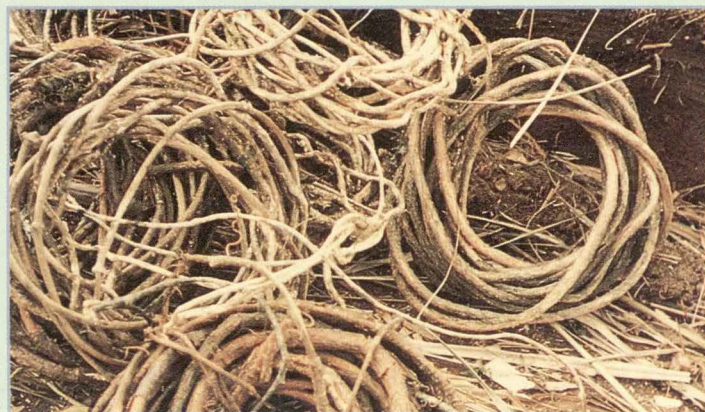
Above Vine ropes used to hold panels.
