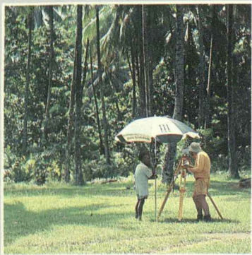
Below Surveyors check dry tilt at Bieng Mission.
