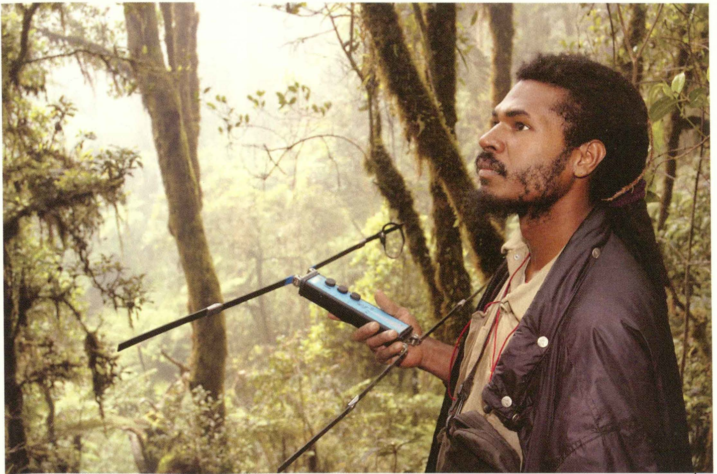
Field scientist Gabriel Porolak uses a radio receiver to track tree kangaroos in the wild.
