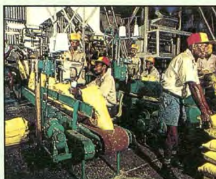
Left: Removing the inner husk in the whitener, producing white rice from brown rice Right: Adding the vitamin enrichment, bagging and tagging the rice for distribution
