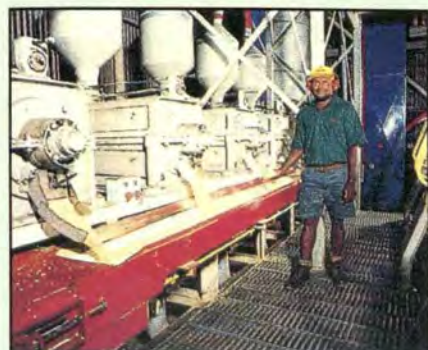
Left: Removing the inner husk in the whitener, producing white rice from brown rice Right: Adding the vitamin enrichment, bagging and tagging the rice for distribution
