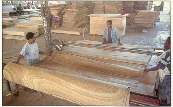
Above: Winding attractive veneer onto rollers as it comes off the knife Below: Carved rosewood table ready for sale
