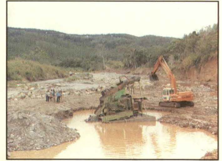
Above: Mechanised alluvial gold mining on the Watut River near Bulolo Below: Loading impure raw gold grain into the acid refining vessels
