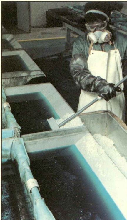
Below: Removal of pure silver crystals from the electro refining cells
