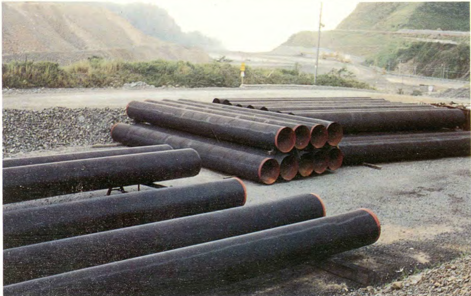
"A portion of a large quantity of steel water supply pipes for Bougainville Copper Ltd., Panguna, externally treated with Dimet Tarsel Standard High Performance Tar Epoxy, to 400 micron dry film thickness. Application by Minenco Pty. Ltd."
