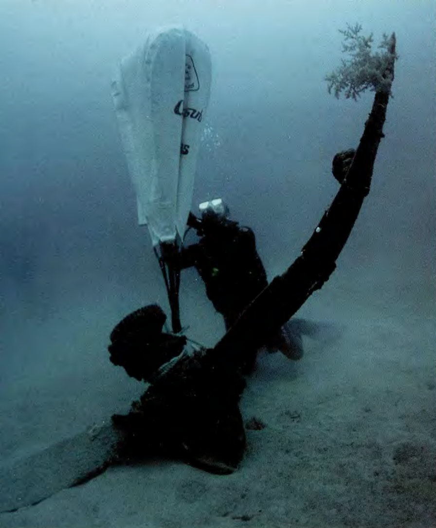
Attaching the lift bag to first propeller.
