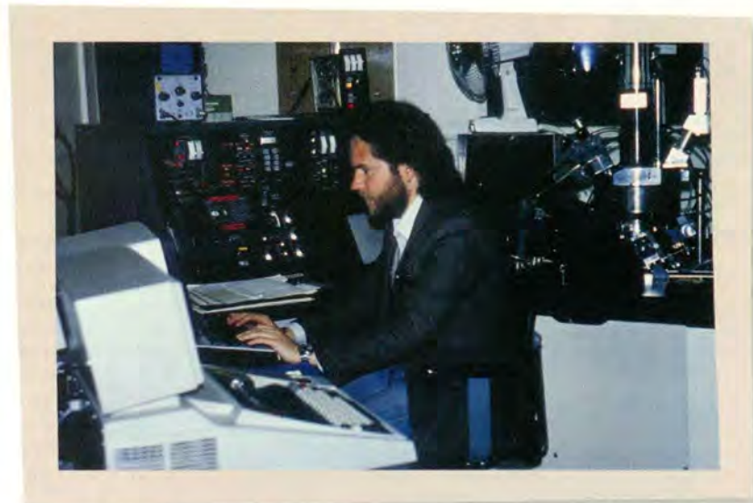
Professor Summerhayes examining chemistry of Lapita pottery using an electron microprobe.
