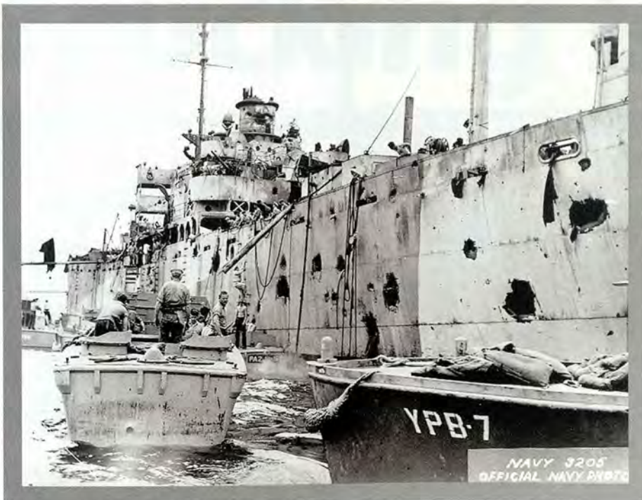
Damage to USS Mindanao from the Mt Hood explosion.
